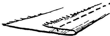
Raw Edge Showing When fed in short, not enough material to fold under.
